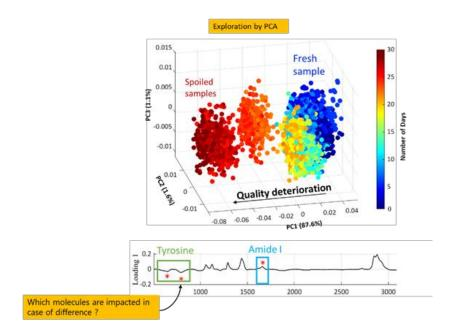
*Figure 13. Raman system capabilities on observing the quality change and detecting the molecules behind this change.*
