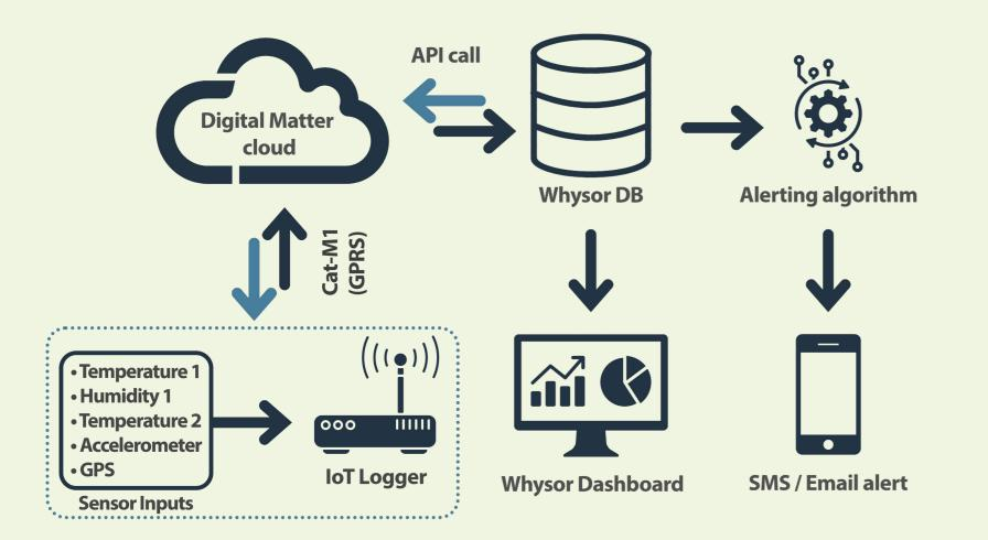
Alerting logic. The threshold values for the alerting system were defined by the logistics and warehouse manager at Musgrave. Text messages are sent when the van is performing a delivery and either the chill zone rises above 5°C, or the freeze zone rises above -8°C. To avoid false alerts, the system records 6 values above the threshold before sending the alert. The values are recorded every 5 minutes by the logger.
