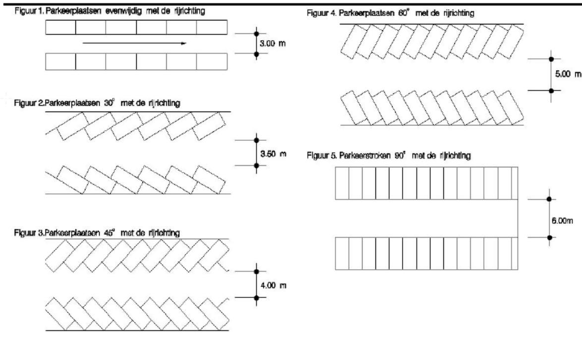
Figure 4: Car parking distances for different angles ([www.leuven.be](http://www.leuven.be))
