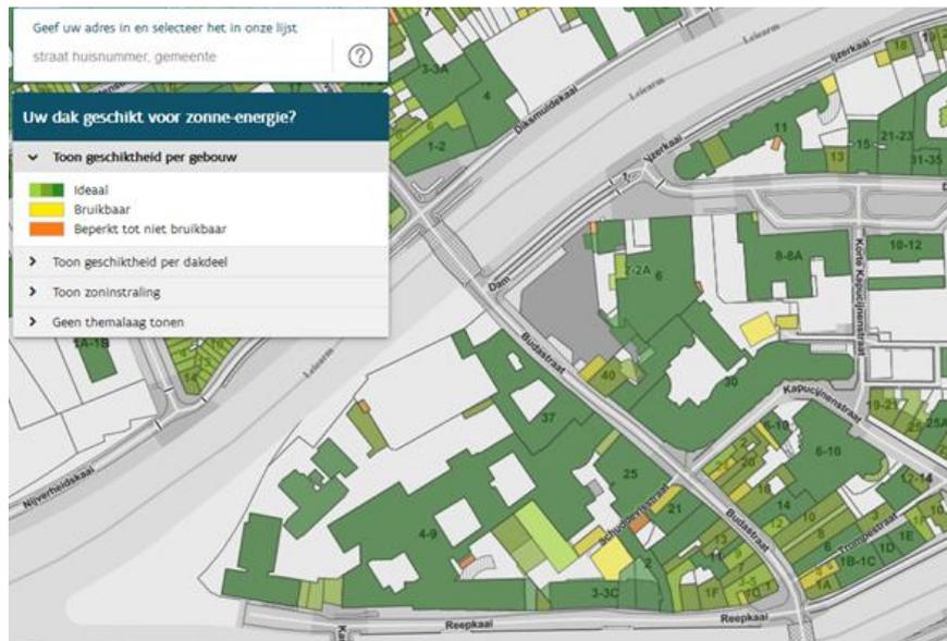
Figure 33: Map showing the relevance of solar panels per building in Kortrijk (Source: Energiesparen)
