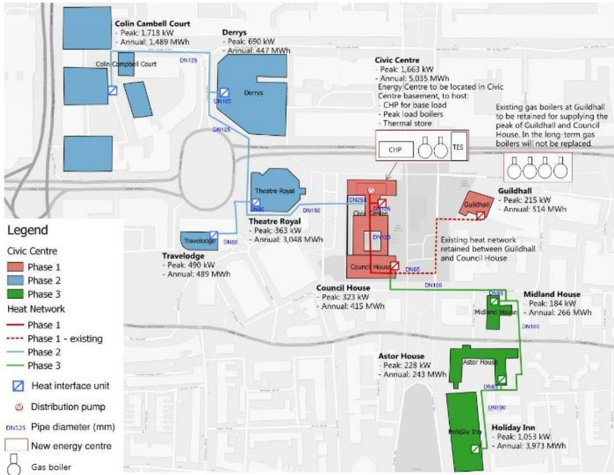
Figure 48: Civic Center scheme (source: Heat mapping and Energy Masterplan, BH)
