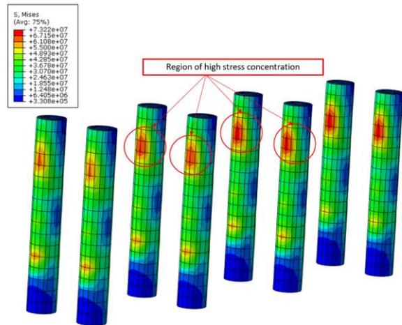
Figure 15: Close-up view showing the region of high stress concentrations of the compressed wood dowels
