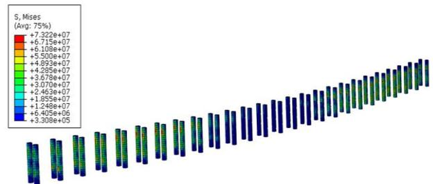
Figure 14: Contour plot showing the stress distribution of the compressed wood dowels
