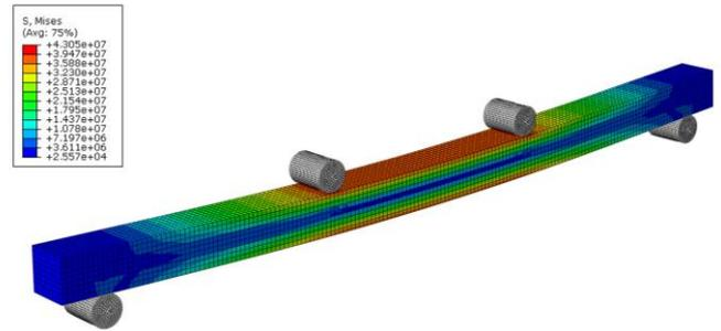
Figure 13: Contour plot showing the stress distribution of the glulam beam (tie constraint)
