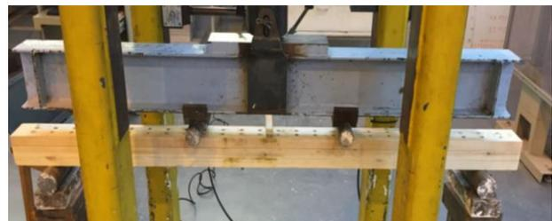
**Figure 9:** AFLT beam setup for four-point bending
