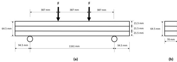
**Figure 6:** The sketches and dimensions of the four-point bending test setup: (a) Side-view and (b) Cross-section view
