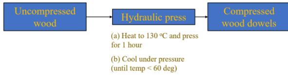
**Figure 1:** An overview of the fabrication processes for the compressed wood dowels
