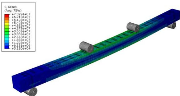
Figure 11: Contour plot showing the stress distribution of the AFLT beam
