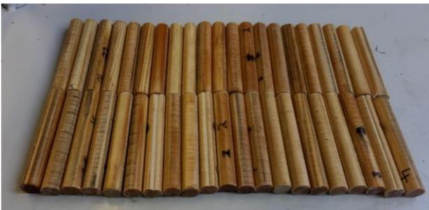
**Figure 3:** A photograph of the compressed wood dowels
