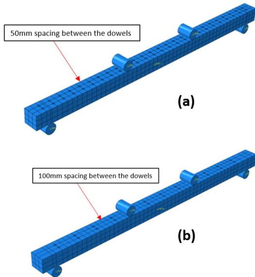
**Figure 16:** Images showing AFLT beams with 50mm and 100mm dowel spacing
