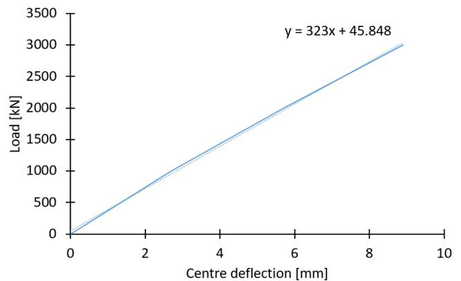
**Figure 18:** Load versus centre deflection plot of the AFLT beam under four-point bending
