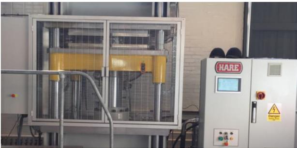
**Figure 2:** A photograph of the 2000 kN hydraulic press used for processing the compressed wood dowels
