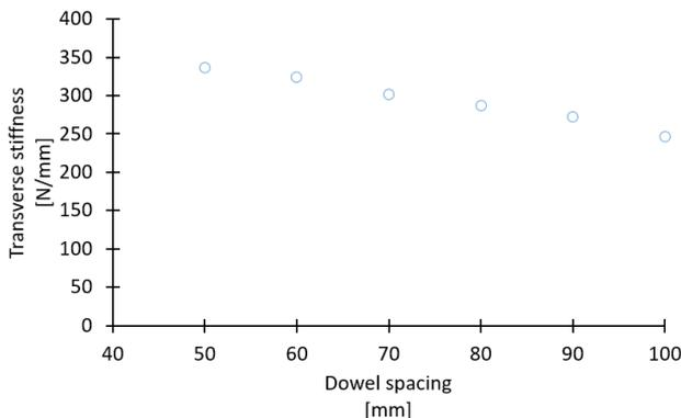
**Figure 17:** A plot of the initial transverse stiffness versus the dowel spacing for the AFLT beam
