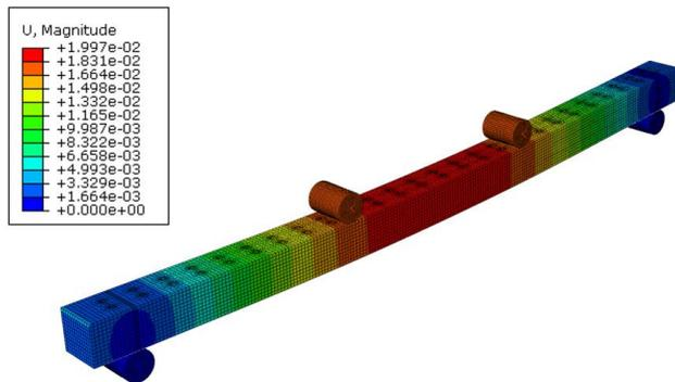
Figure 10: Contour plot showing the deflection response of the AFLT beam
