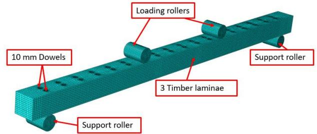
**Figure 8:** Mesh, loading and boundary conditions of the AFLT beam
