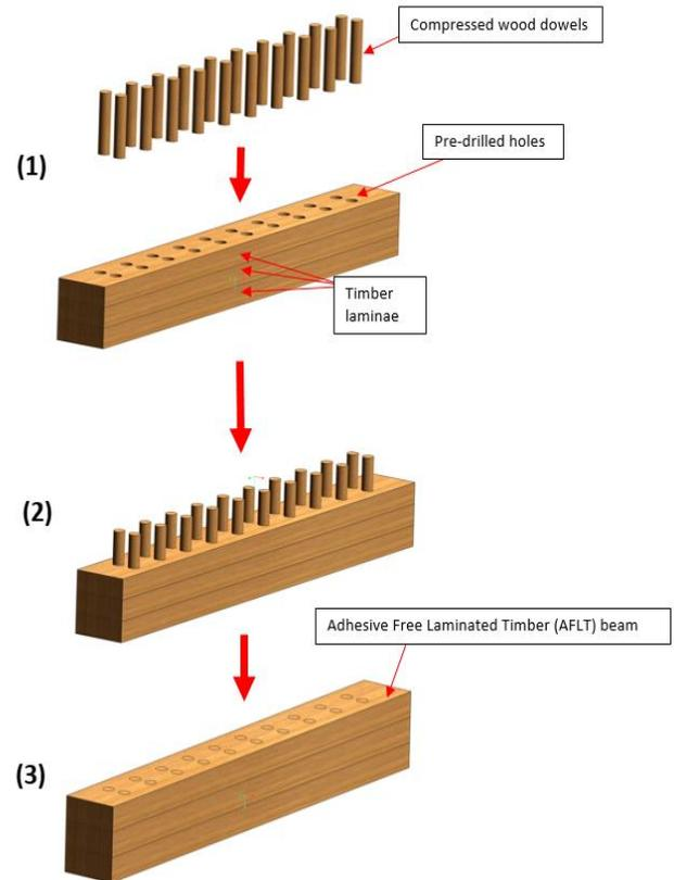
**Figure 4:** Flow diagram showing the assembly processes involved in the fabrication of the AFLT beam
