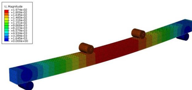
Figure 12: Contour plot showing the deflection response of the glulam beam (tie constraint)
