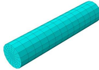
**Figure 7:** Mesh used in the FE model of the compressed wood dowels
