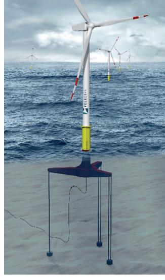
Figure 10: Drawing of an installed tension-leg platform [17]
