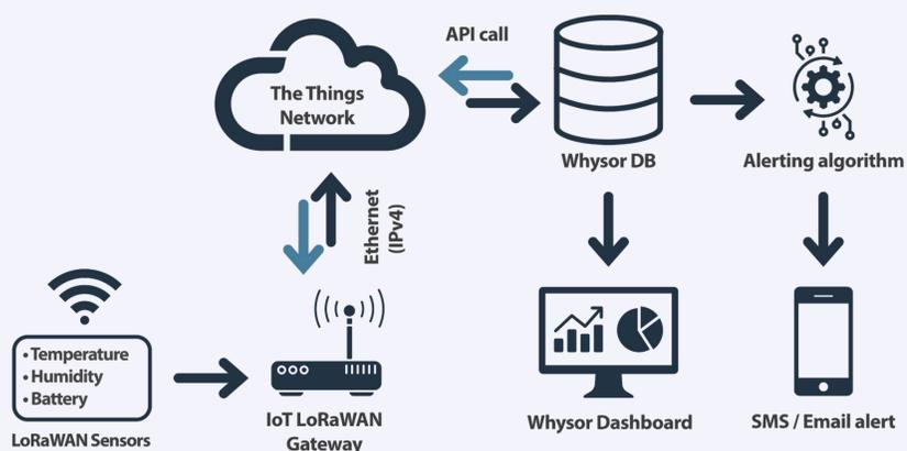
**Alerting logic.** The threshold values for the alerting system were defined by Burns Farm Meats and UCD. Text messages are sent if the temperature in the chambers reach temperatures higher than 7°C.
