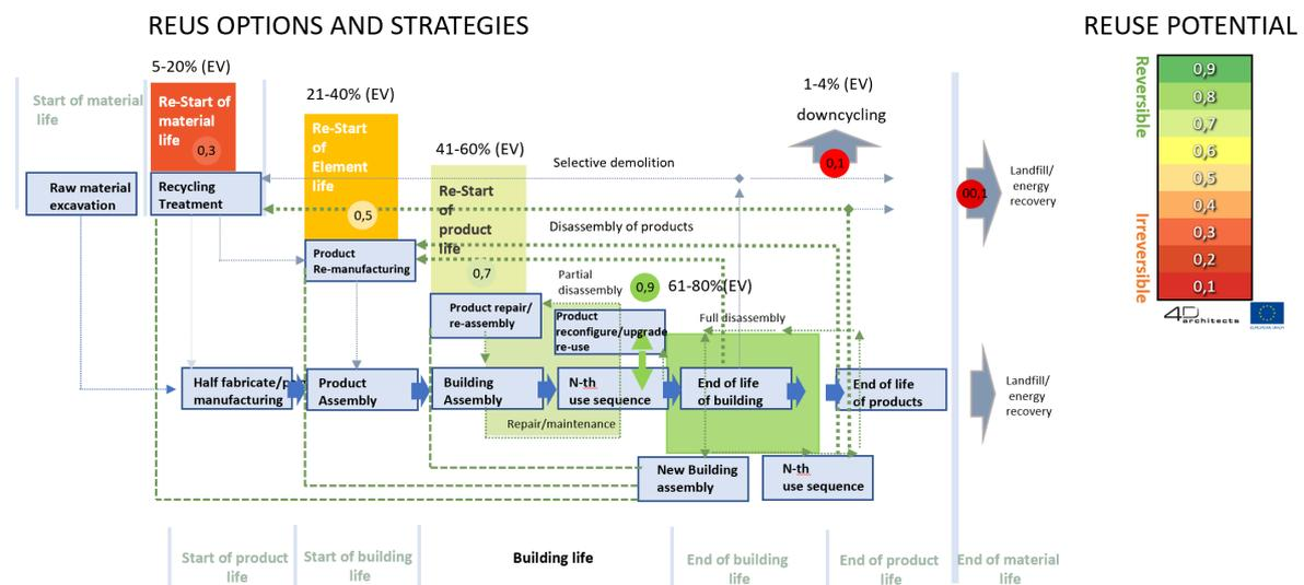
Figure 4. Relation between Reuse Potential score, reuse options of elements (Durmisevic, 2019)
