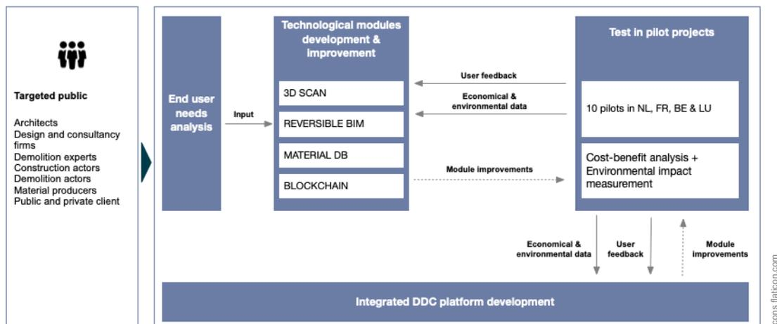
Figure 1. Methodology of for the DDC platform development
