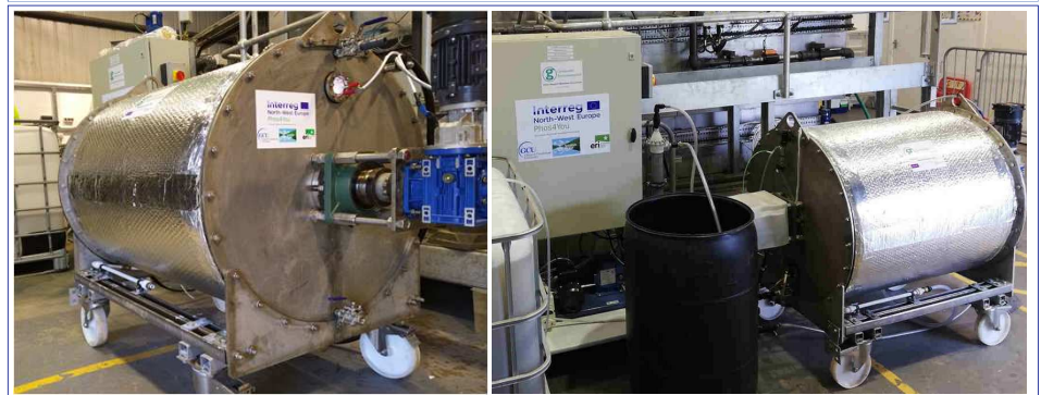
Picture 2: 500L PBR implemented at Bo'ness (© Ania Escudero, GCU)
