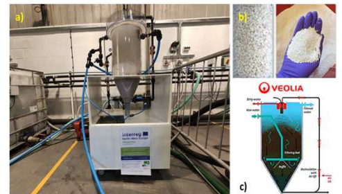
Figure 3: FILTRAFLO™-P reactor designed by Veolia (a and c) and the obtained P-rich CCM material (b) (© Szabolcs Pap, ERI)
