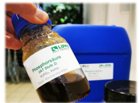
Figure 2: Example for phosphoric acids produced in the "Phos4You" project (© Dennis Blöhse, Lippeverband)
