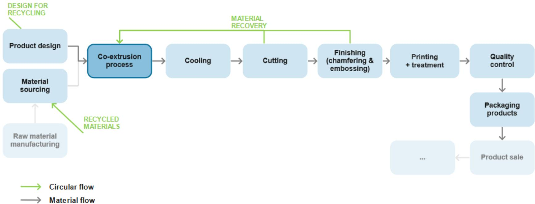
**Figure 5:** Operational process map for Blue Line closures - Vinventions
