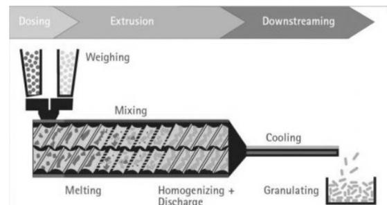
**Figure 6<sup>5</sup>: extrusion principle with twin-screw extruder**
