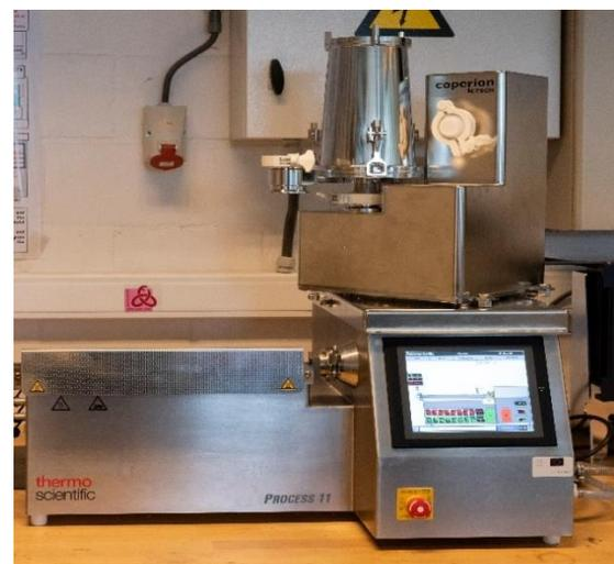
**Figure 7: Process 11 twin-screw extruder from ThermoFisher**
