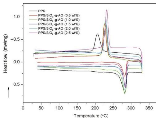
**Figure 5<sup>4</sup>: example of PPS' temperatures transfer depending on nanofillers concentration, observed with Differential Calorimetric Scanning**
