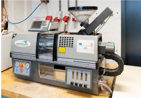
Figure 8: Plastic injection molding from Babyplast
