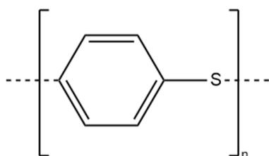
Figure 3: chemical structure of polyphenylenesulfide (PPS)
