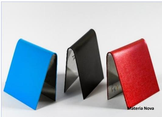
**Figure 4 :** Coloured sol-gel coatings obtained by spray coating on stainless steel. The bending test carried out after coating application and curing shows no cracks on the bended part.
