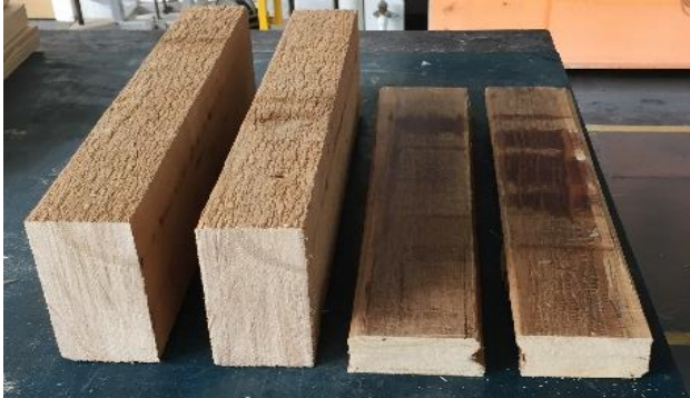
Western Hemlock vertical grain timber sections before and after compression from 400 kg/m 3 to 1400 kg/m 3 . Image by University of Liverpool.
