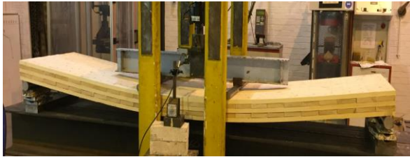
Fig. 4 - Testing of dowelled-laminated floor panel [U Liverpool].
