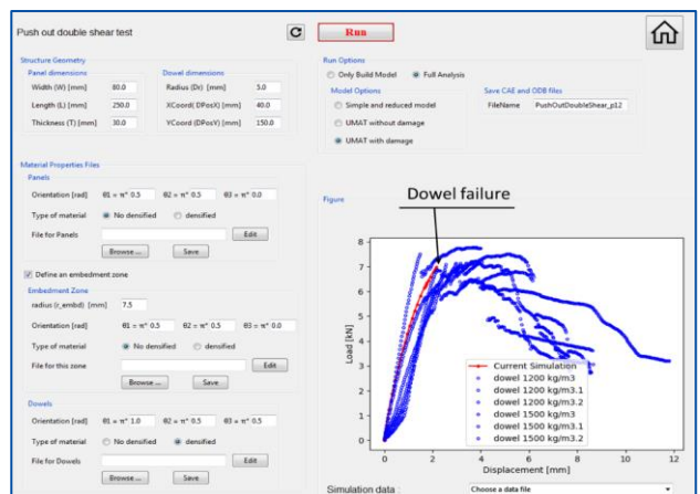
Fig. 11 - User Interface of the numerical results of a push out double shear tests [Luxembourg IST].
