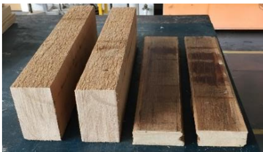
Fig. 1 - Western Hemlock timber sections before and after compression from 400 kg/m 3 to 1400 kg/m 3 [U Liverpool].
