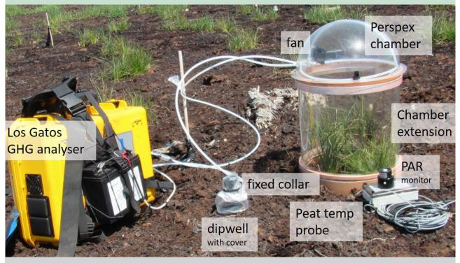
Figure 10. The Greenhouse Gas Monitoring equipment.
