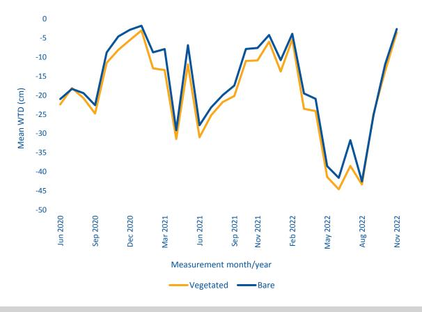
Figure 16. Water table depth (WTD) measurements on the LWM companion planting pilot, showing seasonal variation between monitoring points.
