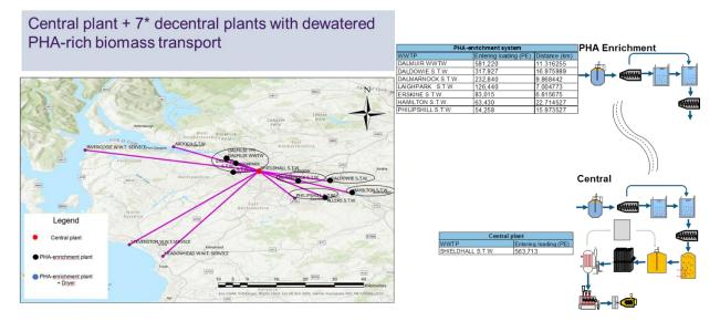
Figure 6-3: variant 2.1 with one central plant and 7 decentral plants providing dewatered PHA-rich biomass
