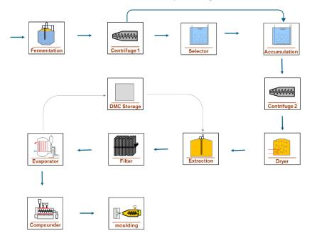
Figure 1-1: Flow diagram of PHA production
