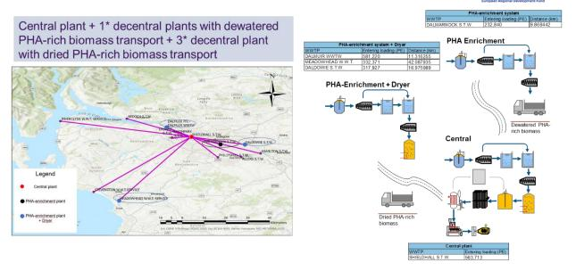
Figure 6-5: variant 3.1 with one central plant, 1 decentral plants providing dewatered PHA-rich biomass and 3 decentral plant providing dried PHA-rich biomass
