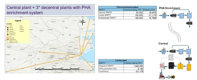
Figure 6-8: variant 1.2 with one central plant and 3 decentral plants providing dewatered PHA-rich biomass
