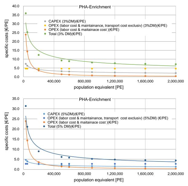
Figure 4-1: specific cost for construction as well as operation a PHA-Enrichment system
