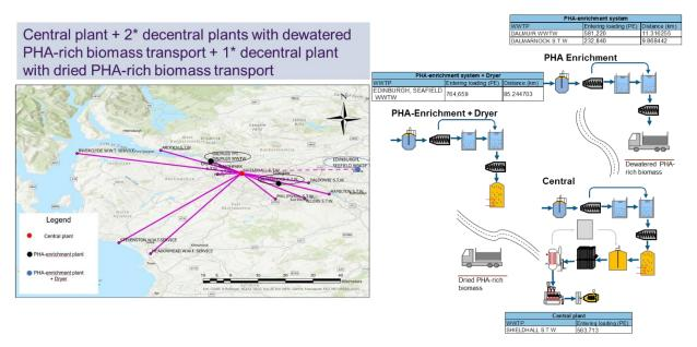
Figure 6-6: variant 3.2 with one central plant, 2 decentral plants providing dewatered PHA-rich biomass and 1 decentral plant providing dried PHA-rich biomass
