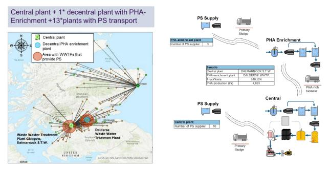
Figure 6-2: variant 1.2 with one central plant and one decentral PHA enrichment plant
