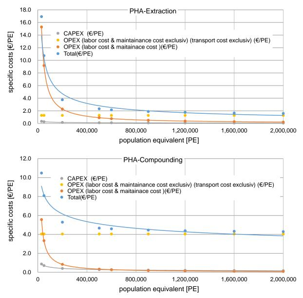
Figure 4-2: specific cost for the PHA-extraction and PHA-compounding system
