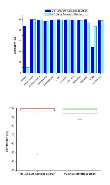
There is not a significative difference in performance between M1 (EmiSure Activated Biochar) and M2 (Wow Activated Biochar)
