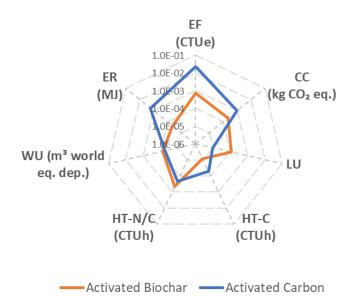
Figure 4.2. Comparison of LCA results for one unit of activated biochar and activated carbon.
