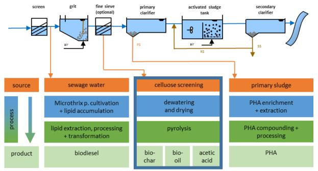
Figure 1.1. Recovery of carbon-based elements from sewage in the WoW! project, with blue highlighted area reflecting biochar production.
