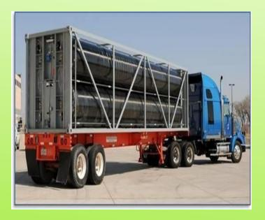
Composite storage vessels with pressure of 700 bar capacities of (**560–900 kg)** of hydrogen per trailer
