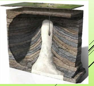
1 Single Cavern Diameter of 50m, height=200m Stored H2= 78M Sm3 (6,500,000 kg) Temp= 290k Pressure= 260 bar
