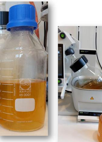
Figure 3. Filtered DMC solution containing extracted PHA. Production from the University of Kaiserslautern-Landau (RPTU)
