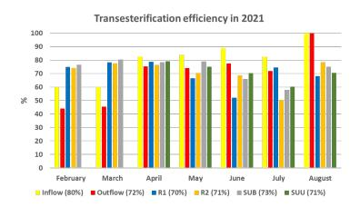
Figure 11. Transesterification efficiency at the Lipid-pilot plant in 2021.
