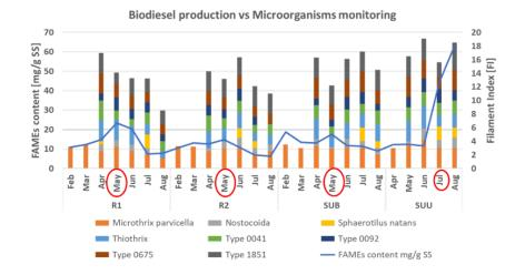
Figure 18. Comparison between Biodiesel production and Microorganisms monitoring in the bioreactors in 2021.
