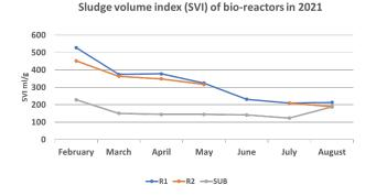
Figure 7. Sludge volume index (SVI) monitoring at the Lipids-pilot plant in 2021.
