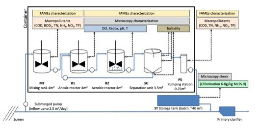
Figure 4. Schematic diagram of the pilot treatment system (Source: University of Luxembourg). The direction of the flow through the individual tanks is indicated by the solid blue lines, and sampling/sensors measurements, by the black dashed lines.
