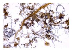
Figure 6. Inoculum with presence of M. parvicella.
