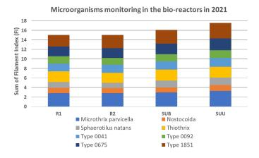
Figure 8. Microorganisms monitoring in the bioreactors at the Lipids-pilot plant in 2021.
