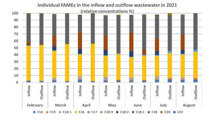
Figure 14. Individual FAMEs from inflow and outflow at the Lipids-pilot plant in 2021.
