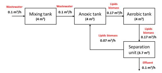
Figure 2. Pilot plant layout
