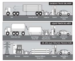
Figure 18: Options for Supplying Hydrogen to a HRS<sup>45</sup>
