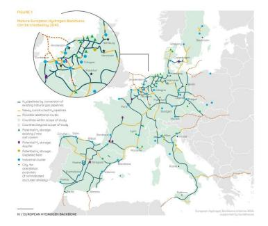
Figure 21: European Hydrogen Backbone 2040 Vision<sup>29</sup>
