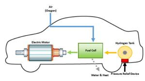
Figure 11: The Hydrogen Fuel Cell Vehicle Concept<sup>40</sup>
